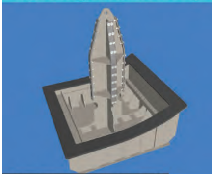
Cofferdam designed using scan data
