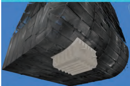
Cofferdam model fitted to FPSO hull scan. Perfect fit is verified before repair begins.
